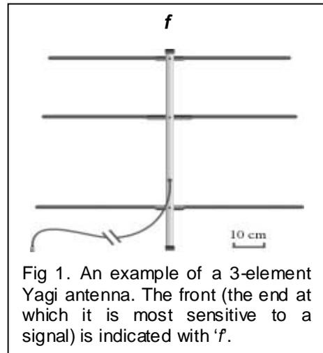
Fig 1. An example of a 3-element Yagi antenna. The front (the end at which it is most sensitive to a signal) is indicated with 'f'.
