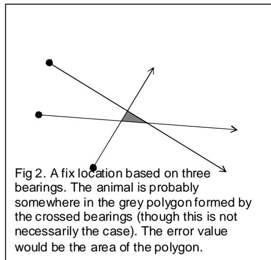
Fig 2. A fix location based on three bearings. The animal is probably somewhere in the grey polygon formed by the crossed bearings (though this is not necessarily the case). The error value would be the area of the polygon.
